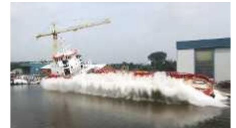
Launch of Wagenborg's IMSV 'Serkeborg'. This transverse launching is a spectacular event which is typical for shipyards in the northern part of the Netherlands.
