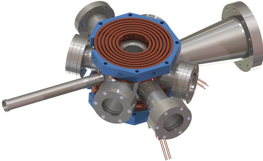
Figure 4.4: The MOT chamber is a simple chamber with 10 ports. The chamber was initially designed for magnetic transport[83] which greatly constrained the vertical dimensions of the chamber.
