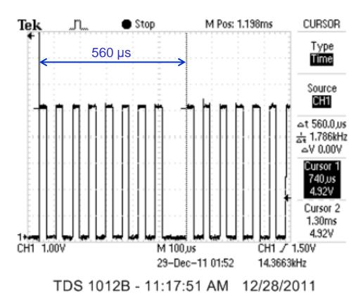
• Transfer rate:  $1/(560 \ \mu s/8 \ bits) = 14.3 \ kbps$
