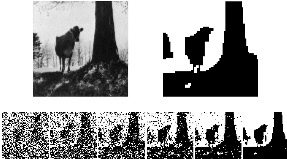
Figure 4: Statistical mechanics can be applied to the segmentation of images. On the top left, a rural scene taken as the external magnetic field, with its intensity scaled so that dark areas are negative, light areas are positive. At the top right, the mode or ground state of the Ising model. Along the bottom, the Gibbs distribution is sampled at a decreasing sequence of temperatures, discovering the global pattern bit by bit.
