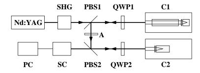
**Figure 3.5:** Experimental setup of double compressor. SHG - second harmonic generation stage, PBS - polarizing beam splitter, QWP - quarter-wave plate, A - attenuator, C - Brillouin compressor, SC - streak camera, PC - personal computer.
