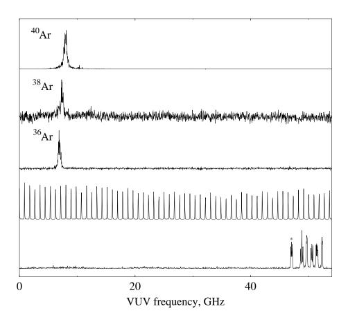
**Figure 6.2:** A scan of the  ${}^{1}S_{0} - 1s_{2}$  resonance for the three isotopes, the etalon markers and the iodine saturation spectrum of R67(9-4). Asterisk (\*) points at the "t" hyperfine component calibrated previously and used as frequency standard at 105 nm.
