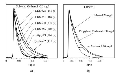
**Figure 7.7:** Fluorescence decay of different dyes measured with a pico-second streakcamera after a femto-second pulse excitation; a) - different dyes in methanol; b) - LDS 751 in different solvents. These measurements were performed with the equipment of the Biophysics laboratory, for which we are grateful to Prof. R. v. Grondelle and B. Gobets.
