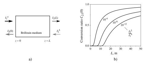
**Figure 1.3:** SBS amplifier; a) - general scheme:  $I_1^{\circ}$  and  $I_2^L$  are the boundary conditions, whereas  $C_{21}(0) = I_2(0)/I_1(0)$  and  $I_1(L)$  are the solutions; b) - the dependence of the conversion ratio  $C_{21}^0$  on the length of a silica fiber (4  $\mu$ m diameter) for different seeding levels and constant (500 mW) pump power.
