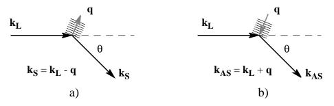
**Figure 1.2:** Spontaneous Brillouin scattering from propagating density fluctuations; a) - spontaneous Stokes scattering at angle  $\theta$ ; b) - spontaneous anti-Stokes scattering.
