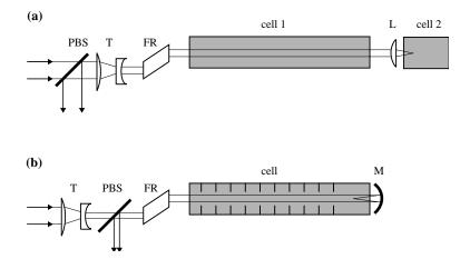
**Figure 2.1:** Geometrical configurations for SBS compressors. a) two-cell compact generator-amplifier setup (CGAS) as used previously by our group [11] with circularly polarized light; b) single-cell geometry used in the present study (T - telescope, PBS - polarizing beam splitter, FR - Fresnel rhomb, L - lens, M - mirror).
