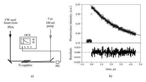
Figure 7.12: Fluorescence decay from the CW seeded pre-amplifier.
