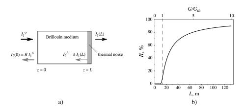
Figure 1.4: SBS generator; a) - general scheme; b) - the dependence of the SBS reflectivity on the length of a silica fiber (4  $\mu$ m diameter) and on the weak-signal gain  $G/G_{th}$  at constant pump power of 500 mW.
