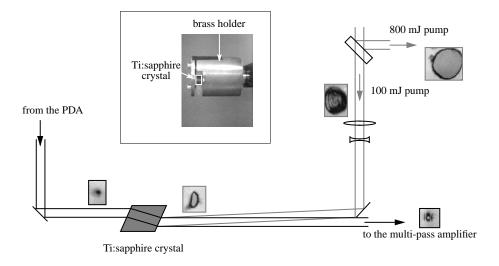
Figure 7.11: Ti:sapphire pre-amplifier setup. The inset shows a photo of the crystal holder. The framed photos show the beam profiles, measured at the respective positions and are in scale.
