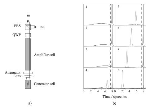
**Figure 1.13:** Two-stage generator-amplifier setup; a) - Experimental arrangement: PBS - polarization beam-splitter, QWP - quarter-wave plate; b) - A time sequence of the modeled pulse compression by SBS in focusing geometry. The evolution stages of the compression follow the Arabic numerals.
