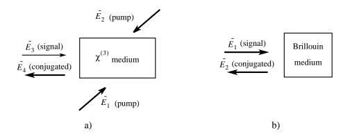
Figure 1.10: Phase conjugation; a) - by degenerate four-wave mixing, b) - by SBS.
