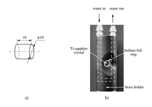
Figure 7.15: The Ti:sapphire multi-pass amplifier crystal; a) - crystal dimensions; b) - the crystal holder design.
