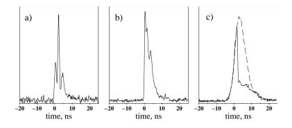
**Figure 4.4:** Typical temporal pulse shapes: a) backward scattered pulse; b) forward scattered second Stokes; c) pulse shape in the forward ring - the outer part (solid line) takes part in the stimulated scattering, whereas the inner part (dashed line) is not affected by the interaction.
