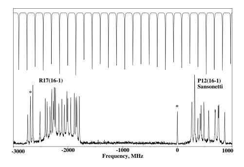
**Figure 5.2:** Simultaneous scan over two lines (R17 and P12) in the *B-X* (16-1) band of I<sub>2</sub> (lower trace) and the fringes of a stabilized etalon (upper trace). The "t" components are denoted by \*. Note that for the R(17) line all 21 transitions corresponding to  $\Delta F = \Delta J = +1$  are resolved.
