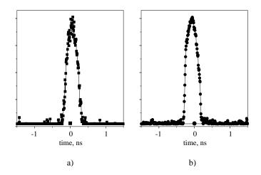
**Figure 7.10:** Pulse duration measurements with a streak camera; a) - the pump pulse from the SBS pulse compressor  $\tau_{SBS} = 337$  ps; b) - the output pulse of the PDA  $\tau_{PDA} = 358$  ps. The widths are measured at 1/e level.
