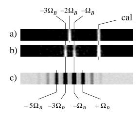
**Figure 4.3:** Spectra, recorded by the grating monochromator: a) - central spot in forward direction where second Stokes frequency is visible; b) - backward scattered beam with third and first Stokes frequencies; c) - four-wave-mixing inside the fiber used as a 'ruler' for the relative frequency measurements. The line, denoted by *cal.* is a reference frequency.
