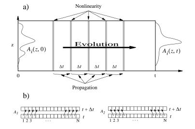
Figure 3.3: The split-step method; a) - the action of the propagation and the nonlinearity operators is split in time; b) - the action of the propagation operator is simply a shift in the discretization bins of the the two fields ( $A_1$ -laser,  $A_2$ -Stokes) if  $\Delta z = c\Delta t/n$ .
