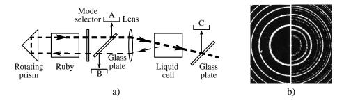
**Figure 1.6:** Higher order SBS experiment in liquids [12]; a) - experimental setup; b) - Fabry-Perot interferograms from site A with water in the liquid cell. Left: below threshold for SBS. Right: above threshold with three Brillouin components in addition to the original laser frequency.
