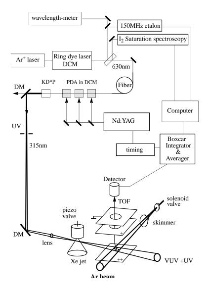
Figure 6.1: Scheme of the experimental setup.
