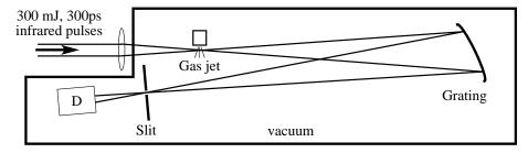
Figure 7.18: The harmonic order separation and detection setup.
