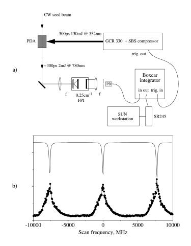
**Figure 7.8:** Spectral characterization of the PDA output. a) - Scheme of the experiment; b) - transmission peaks of the CW seeding (upper trace *inverted*) and the PDA output (lower trace) through a  $0.25 \text{ cm}^{-1}$  Fabry-Perot interferometer.
