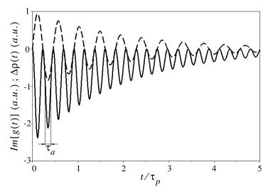
Figure 3.2: Imaginary part of the gain function g(t) (solid line) and the acoustic field  $\Delta \rho(t)$  (dashed line) generated by a short  $\delta$ -like pulse in water for  $\lambda = 532$  nm. Note that the ratio  $\tau_p/\tau_a$  is a material property.
