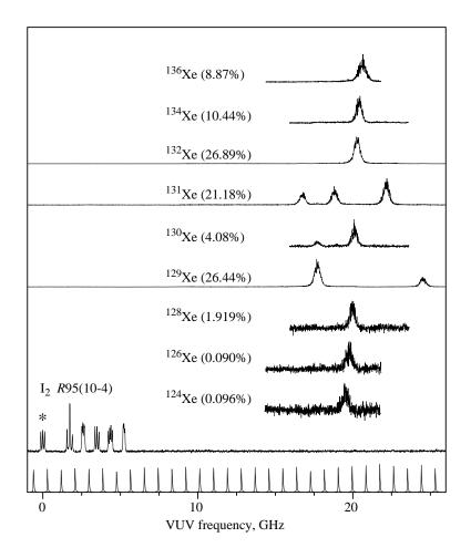
**Figure 6.4:** Spectra of the  $(5p^6 - 7s'[1/2]_1)$  transition, for all natural isotopes of Xenon. FPI transmission peaks, from which the frequency scale is deduced are also shown. The zero frequency is the "t" hyperfine component of R95(10-4) I<sub>2</sub> line (\*) used for absolute frequency calibration.
