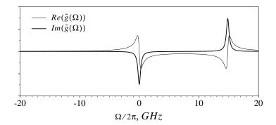
Figure 3.1: Real (thin line) and imaginary (thick line) parts of the SBS gain calculated for water at  $\lambda = 532$  nm. The Stokes shift is  $\Omega_B/2\pi = 7.42$  GHz. The Brillouin line-width is  $\Gamma_B = 539$  MHz
