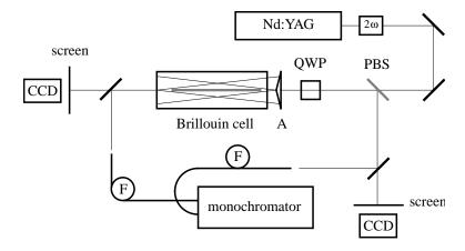
**Figure 4.1:** Scheme of the experimental setup: PBS - polarization beam-splitter; QWP - quarter wave-plate; A -  $2.5^{\circ}$  quartz axicon; CCD - CCD-camera for beam profile recording; F - bare-tip single-mode fiber. A double fiber-input monochromator is used for frequency measurements.
