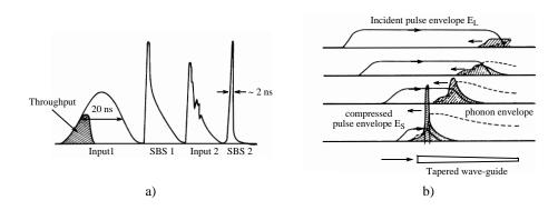
**Figure 1.12:** Pulse compression by SBS [44]; a) - Input, throughput, and SBS signals in two-step pulse compression; b) - Time sequence of SBS compression of a square incident pulse in a tapered wave-guide.
