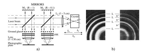
**Figure 1.5:** First experimental observation of stimulated Brillouin scattering [10]; a) - schematic of the experimental arrangement, b) - Fabry-Perot interferograms of the laser radiation (rings labeled L) and of the Brillouin scattered radiation (rings labeled B).
