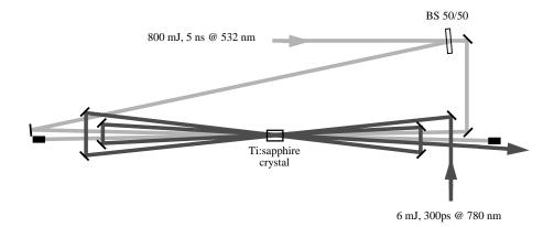
Amplification stage Harmonic generation geometry  $10^{15}$  $10^{14}$ Peak intensity, W/cm<sup>2</sup>  $10^{13}$  $10^{12}$  $10^{11}$  $10^{10}$  $10^{9}$  $10^{8}$  $10^{7}$ Ti:sapphire Ti:sapphire multi-pass PDA Hollow fiber Gas jet Bessel beam pre-amplifie amplifier Beam  $5 \mathrm{mm}$  $5 \mathrm{mm}$ 60 µm  $8 \mathrm{mm}$ 20 µm diameter Energy  $2 \mathrm{mJ}$ 300 mJ 300 mJ 300 mJ 300mJ 6 mJ per pulse
