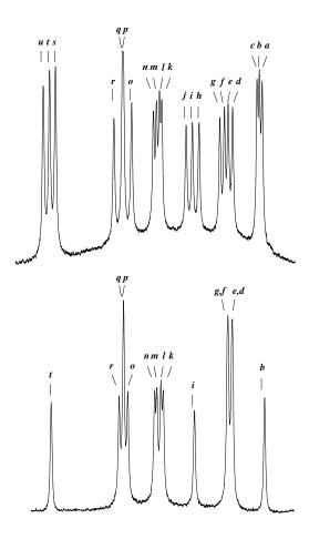
Figure 5.3: Typical pattern of hyperfine structures in I<sub>2</sub>. The upper trace is a recording of the R69(16-1) line and shows the typical structure for an odd-J line with 21  $\Delta F = \Delta J$  main transitions. The lower trace shows the R98(16-1) line with the typical 15  $\Delta F = \Delta J$  main transitions in an even-J line. In the present study we have adopted the identification of "a"-"u" components of Sansonetti [20].
