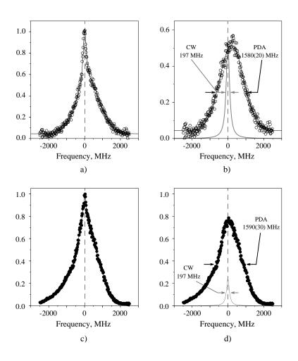
**Figure 7.9:** Spectral characterization of the PDA output; a) - an average over 20 transmission peaks (the data points) and a fit (*see* the text for details); b) - the CW contribution (the gray line) and the PDA transmission peak, fitted with a Gaussian function.
