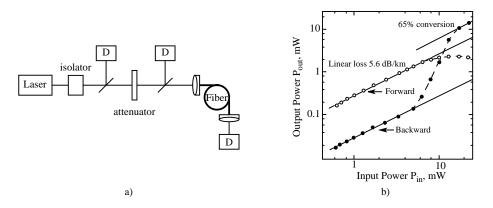
**Figure 1.8:** SBS in optical fibers [28]; a) - experimental setup, b) - transmitted ( $\circ$ ) and reflected ( $\bullet$ ) powers as a function of the input power launched into a 13.6 km long single-mode fiber.
