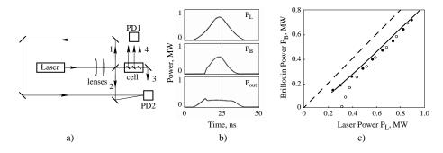
Figure 1.7: SBS experiment in the time domain [24]; a) - experimental setup, b) - oscilloscope traces of the laser power  $P_L$ , the SBS power  $P_B$ , and the transmitted laser power  $P_{out}$  in ethyl ether; c) - instantaneous Brillouin power  $P_B$  versus rising ( $\circ$ ) and falling ( $\bullet$ ) instantaneous laser power  $P_L$  in a cell of 50 cm length filled with ethyl ether. The solid line is a calculation, while the dashed line represents 100% conversion efficiency.
