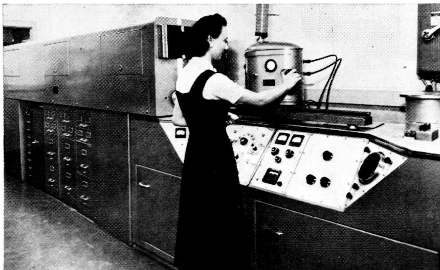
Emission Spectrograph for analysis of raw materials, Marshall St. Laboratories, North Adams, Mass.
