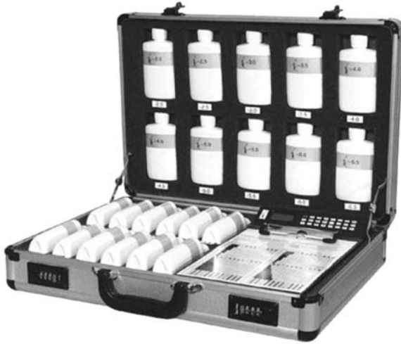
Figure 13.1 An example of a commercially-available detection threshold test kit. In this test, standardised forms are used with randomised presentation orders to present stimuli in a single staircase (SS) procedure. Environmental temperature is recorded, and the geometric mean of the last of four staircase procedures serves as the threshold estimate. Photograph courtesy of Sensonics, Inc., Haddon Hts., NJ, USA.
