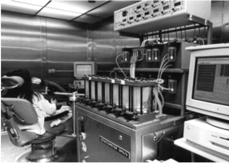
Figure 13.2 A modern air-dilution olfactometer, the Burghard OMB-4, a device that presents odors to the nasal chambers at well-defined quantities and durations. Left: Subject being presented with odors and performing a computerized visual attention task. Right: Data collection module. Center: olfactometer body. Photo courtesy of the University of Pennsylvania Smell and Taste Center, Philadelphia, PA, USA.
