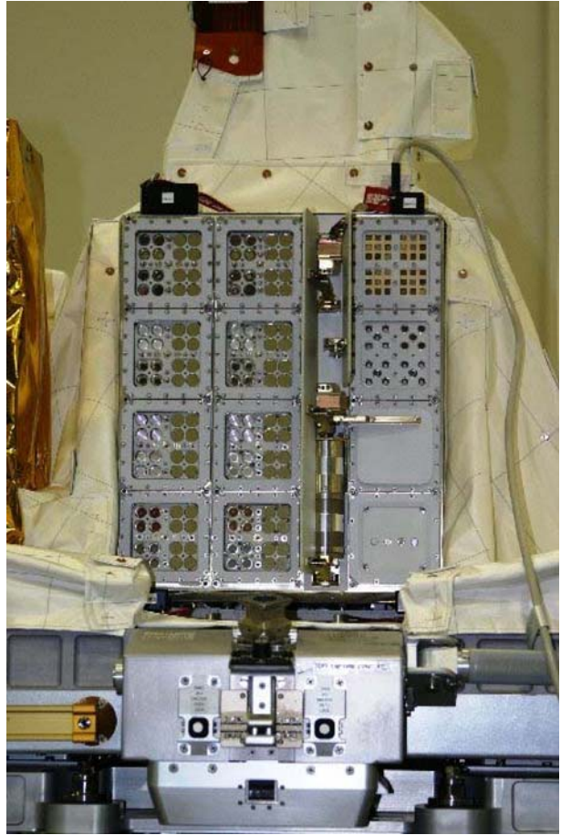
Fig. 4 EXPOSE-E facility mounted on the EuTEF platform during pre-flight tests on ground (courtesy Ralf von Heise-Rotenburg, KT)
