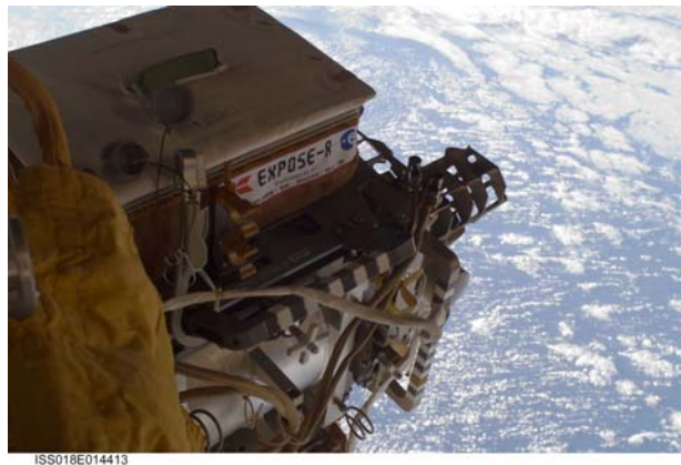
Fig. 6 EXPOSE-R temporarily attached to the URM-D platform of the Russian module Zvezda on 23 December 2008, with protecting cover (Credit: ESA and NASA)
