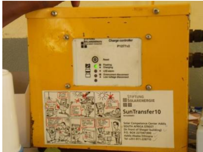
Picture 14: A user friendly short manual on the power box teaches the user how to use the SHS.
