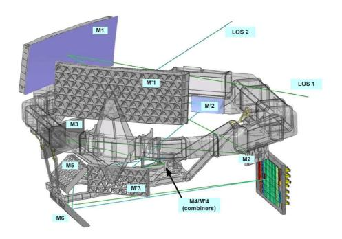
The optical path of both telescopes is composed of six reflectors (M1–M6), two of which are common (M5–M6). The entrance pupil of each telescope is 1.45 m  $\times$  0.5 m<sup>2</sup> and the focal length is 35 m. The payload module features a common focal plane shared by both telescopes. Figure courtesy of EADS-Astrium.
