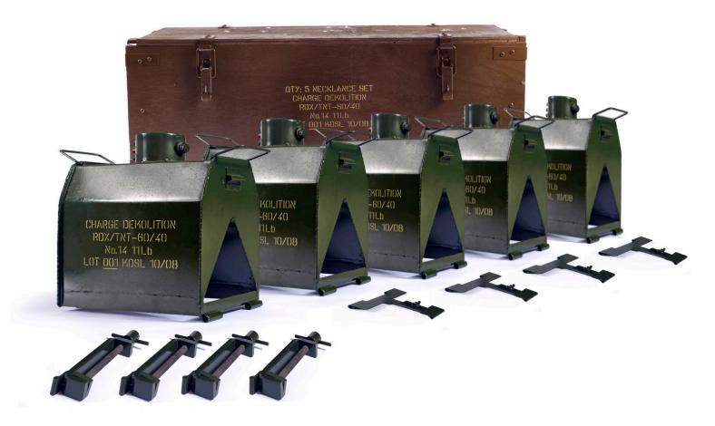
Charge Demolition Necklace L1A1, is a set of 5 "Hayrick" steel vee-linear cutting charges (11lb). Typically used by military Engineers for use against re-inforced metal/concrete targets such as bridge girders. Each of the 5 charges comprises a linear shaped charge unit filled with 5.3 kg of high explosive Composition B "Comp B" (RDX/TNT) primed with a powerful HE booster unit to ensure good performance.
