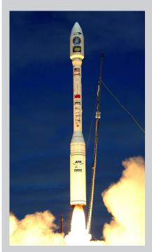
The Taurus launch vehicle is a ground-launched variant of Orbital's highly successful Pegasus<sup>®</sup> air-launched space booster.
