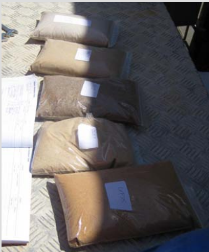
Various sands used to obtain pointing mixes that match original mortars.
