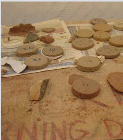
Samples of various synthetic stone mixes trialled using different sands.
