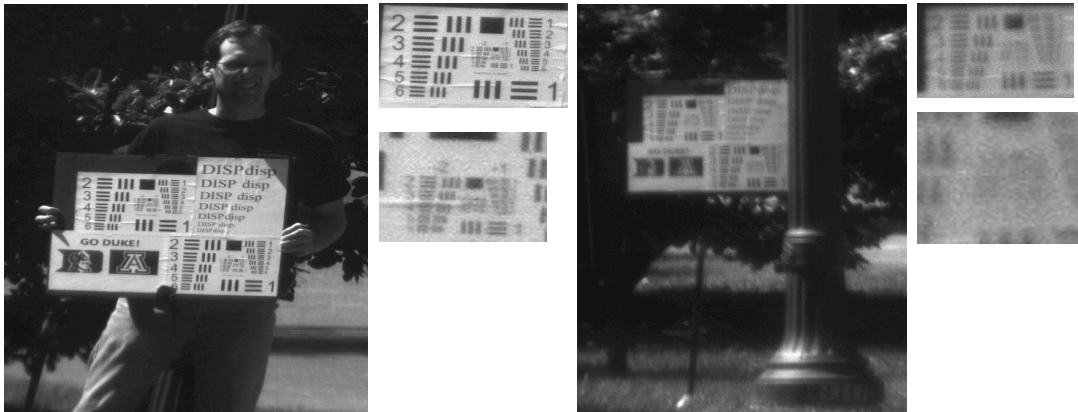
Figure 3. Resolution target captured at 66 meters by AWARE 10 optics (left) and AWARE 2 (right), with zoomed details for each.
