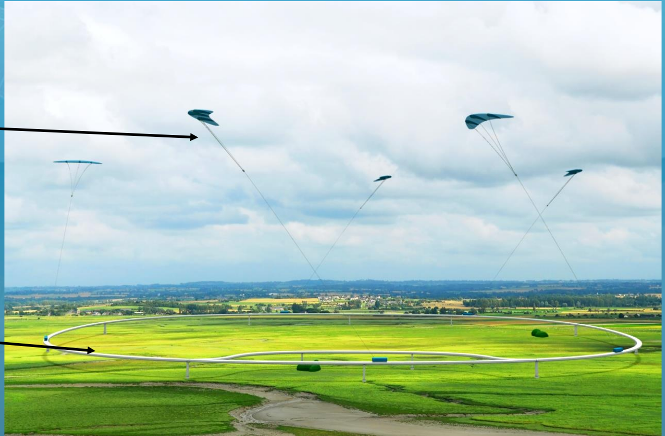
Simulation of an X-Wind plant
