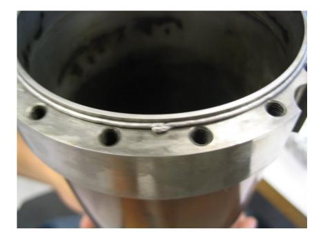
Fig. 7: Insert without inner radiation shield
