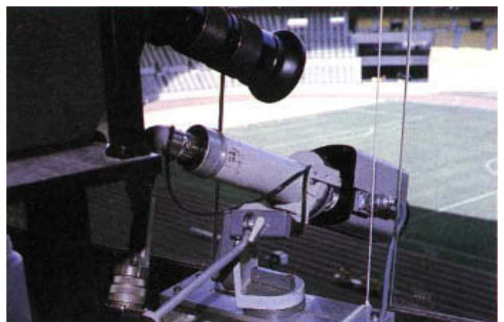
Photo-finish equipment with a backup videotape system was used to decide close results in cycling in the velodrome.
