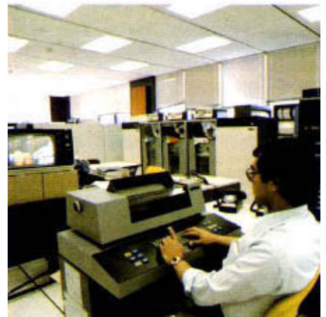
The results centre computer received results and start lists by telephone data lines and retransmitted them to press centres.
