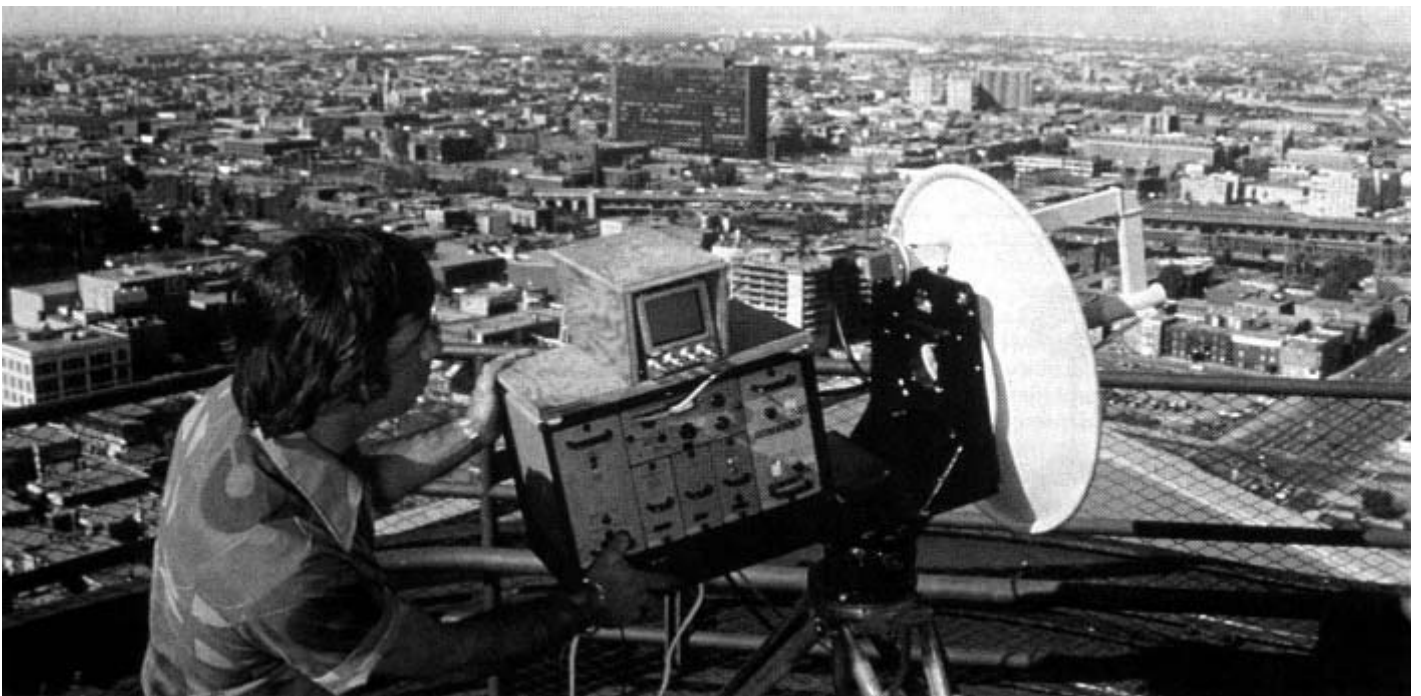
A parabolic antenna on the roof of Maison de Radio-Canada picked up microwave retransmissions of pictures and sound from helicopters and camera cars.
