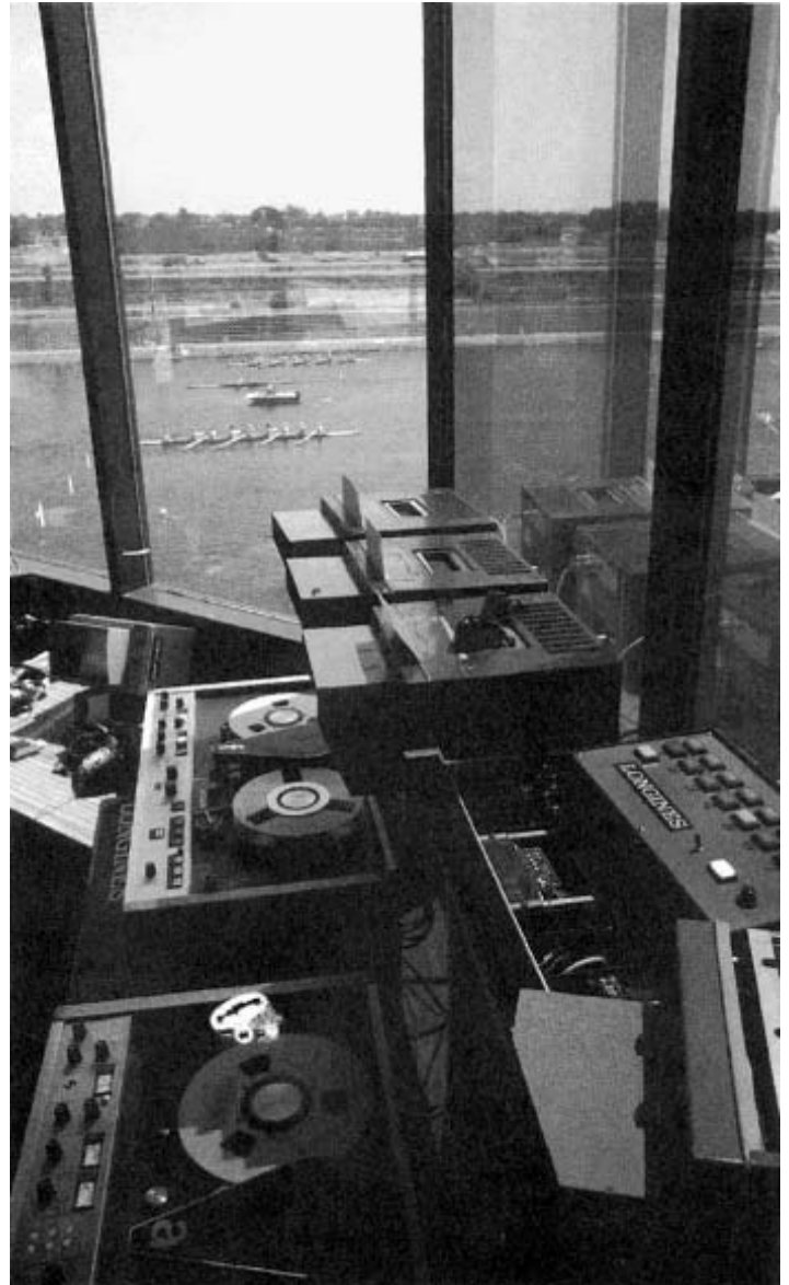
Video timing control equipment for rowing in the photo-finish tower at the Olympic Basin, Notre Dame Island.
