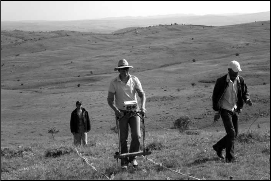
Fig.4: Electrical resistance survey of the 'Temple' area by a team of three.
