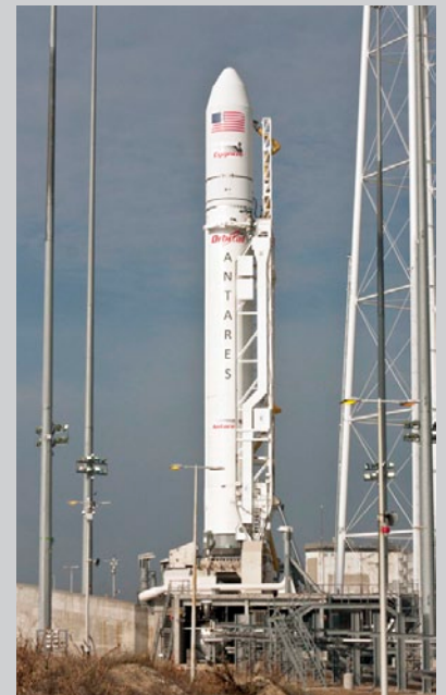
Cygnus is boosted into orbit by Orbital's Antares™ medium-class space launch vehicle.
