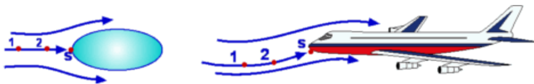
Figure 23 : Stagnation Point on (a) Simple Body and (b) a complicated Body
