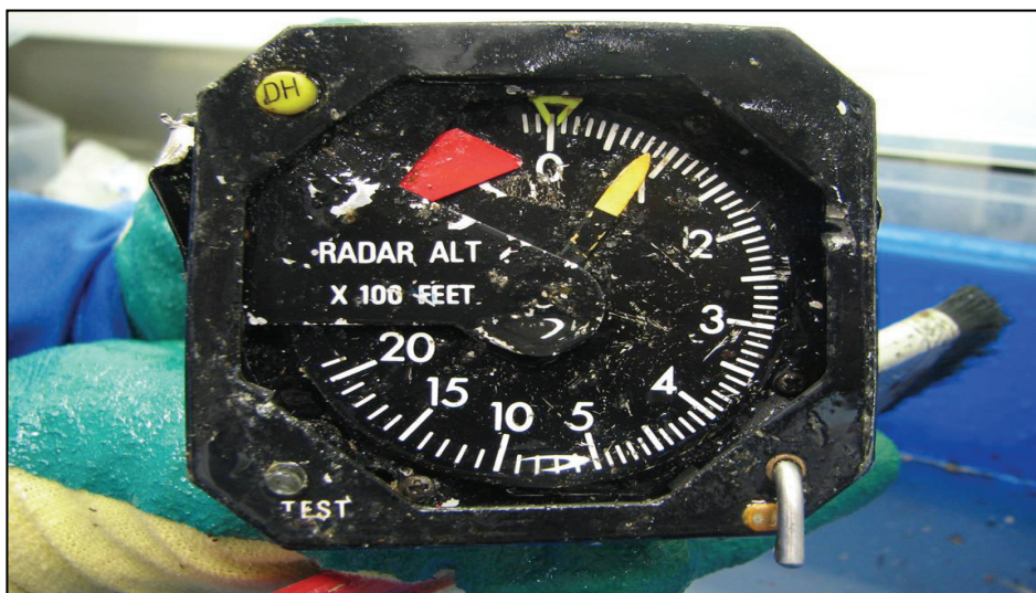
Figure 12: Radar altimeter instrument
