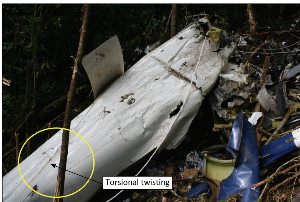
Figure 11: Aft section of the main fuselage showing torsional twisting
