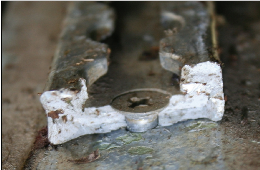
Figure 14: Exemplar overload failure of seat track
