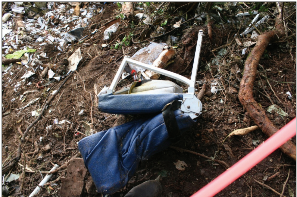
Figure 15: Distorted passenger seat with seat belt attached
