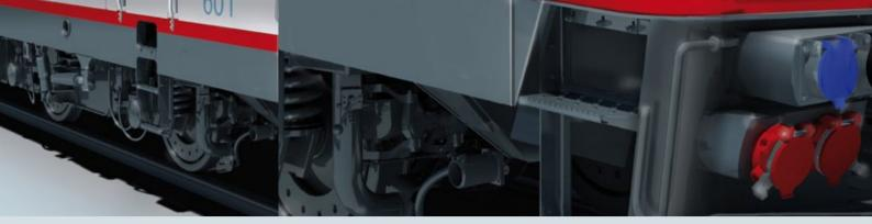
The propulsion unit consists of a pinion hollow shaft drive with the traction motor mounted directly to the truck frame by rubber elements. The gear is axle mounted riding on the wheel set with the other side mounted to the motor case by a reaction rod.
