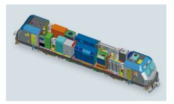
The carbody is designed to allow compression forces up to 3,5 MN (buff load = 800,000 lbs). It is equipped with a Crash Energy Managment (CEM) system that provides enhanced safety for the crews, consisting of an AAR F-Type coupler with pushback mechanism and crash elements.
