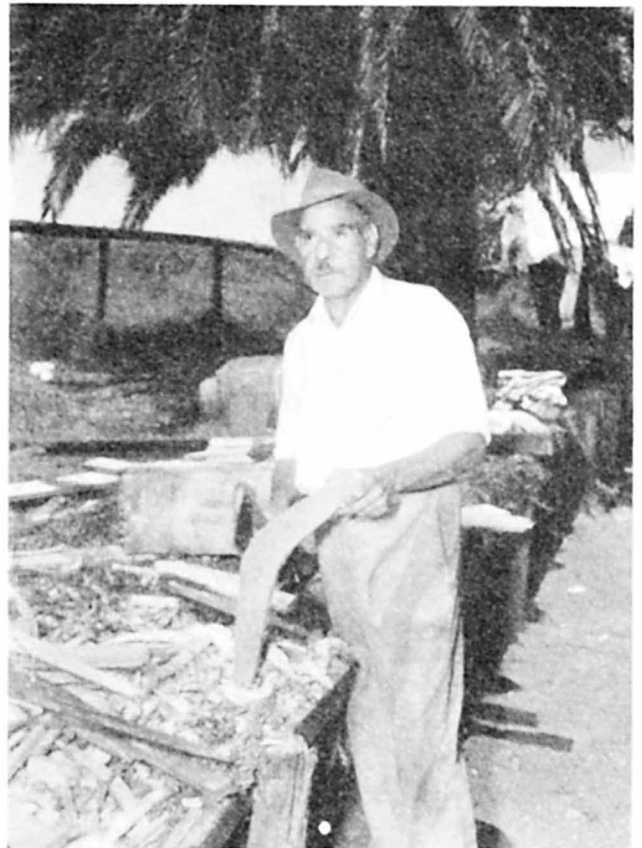
The chips fly as Bob Simms shapes a boomerang from a white mangrove stick—the best timber for the purpose—at his La Perouse workshop
