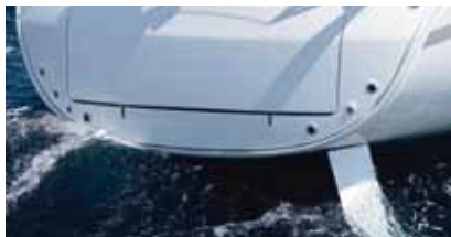
Twin rudders with the CR 56, 50 and 46
