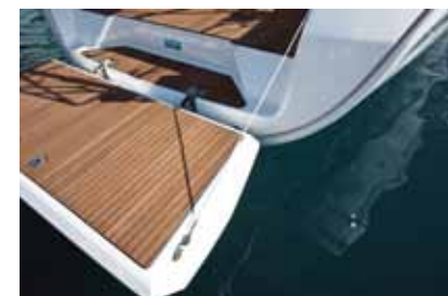
Bathing platform spans the entire width of the stern
