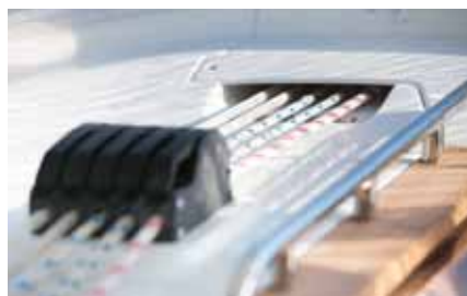
All halyards and lines are led directly into the cockpit (ill. CR 41) for easy and centralised handling
