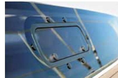
Flush-mounted portlights in the side windows
