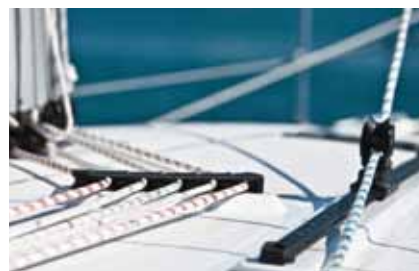
The genoa tracks are positioned on top of the coach roof, ensuring uncluttered decks as well as excellent up-wind characteristics
