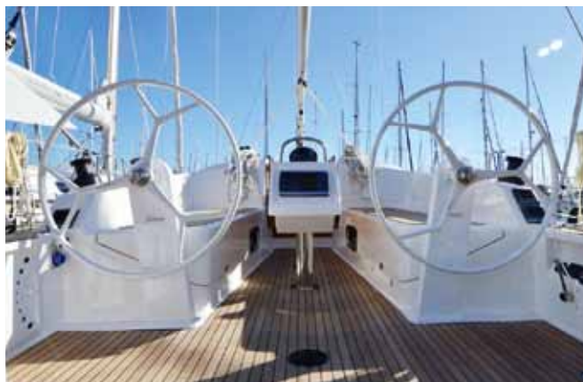
The twin-steering system of the CR 56, 50, 46, 41 and 37. Good cover through high spray hoods* and complete biminis* against wind and weather
