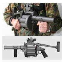
The Milkor 40mm Multiple Grenade Launcher Mk1L is a third generation improved MGL and features an extended 140mm cylinder to accomodate special rounds for lethal and less-lethal applications.
