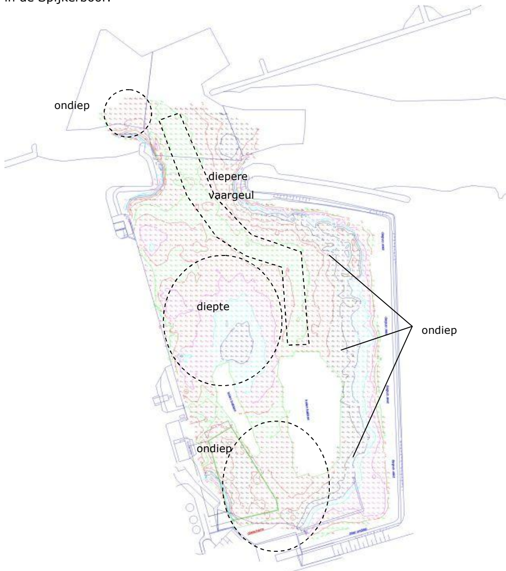
Figuur 3-2 Bodempelling industriehaven Amercentrale, april 2005
