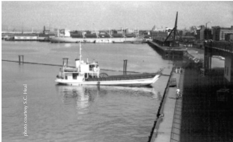
The Coal Island was one of the early vessels in Shields Navigation's fleet. Note the cable-laying drum just forward of the wheelhouse.
