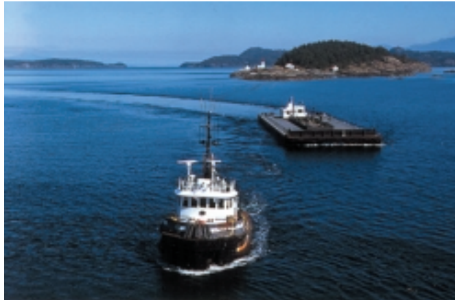
The 59-foot, 1050-horsepower Island Wave (1977, Allied Shipbuilders) one of ITB's coastal tugs, with the 23,000 barrel tank barge Empire 45 .
