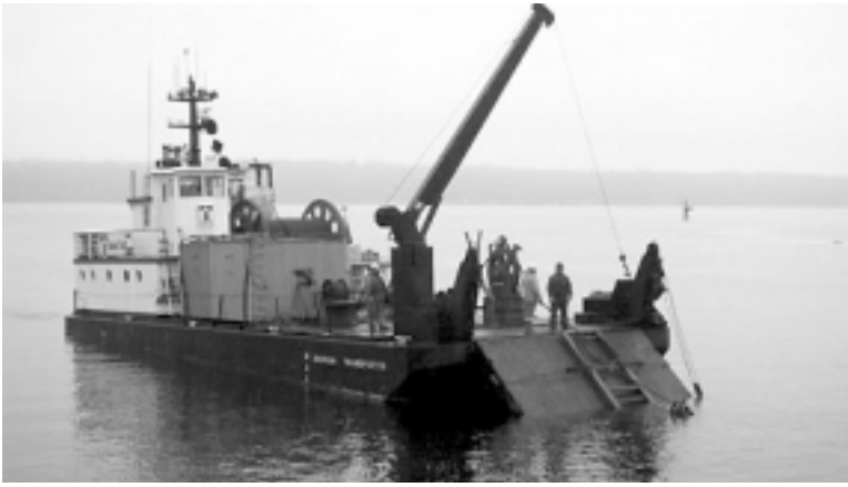
The Georgia Transporter (1963, Mckenzie Barge & Derrick) is a self-propelled cable-laying ramp barge, used by Island Tug and Barge to service its continuing contracts with Telus and BC Hydro, as well as other cable-laying projects.
