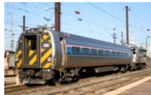
Figure 14: Cab Car Used for Push-Pull Operations
