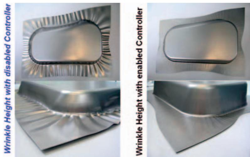
**Fig. 5:** Left: Hishida part geometry with disabled wrinkle height limiting controller.
