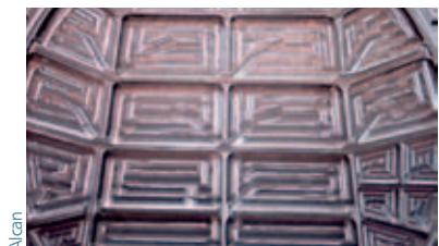
"Machined bulkhead" for Eclipse model 500 aircraft
