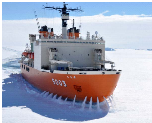
Fig.1 Ramming operation with water flushing
