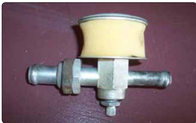
Figure 10-89. A vacuum regulator, also known as a suction relief valve, includes a foam filter. To relieve vacuum, outside air of a higher pressure must be drawn into the system. This air must be clean to prevent damage to the pump.
