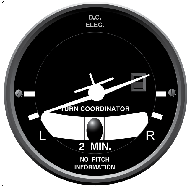
Figure 10-104. A turn coordinator senses and indicates the rate of both roll and yaw.
