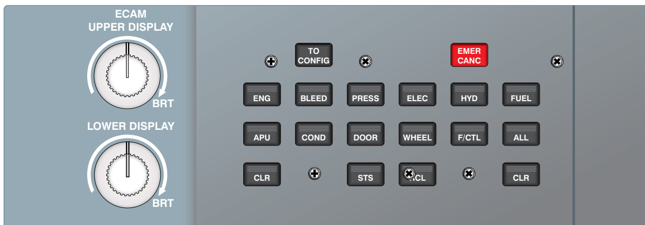
Figure 10-121. An ECAM display control panel.
