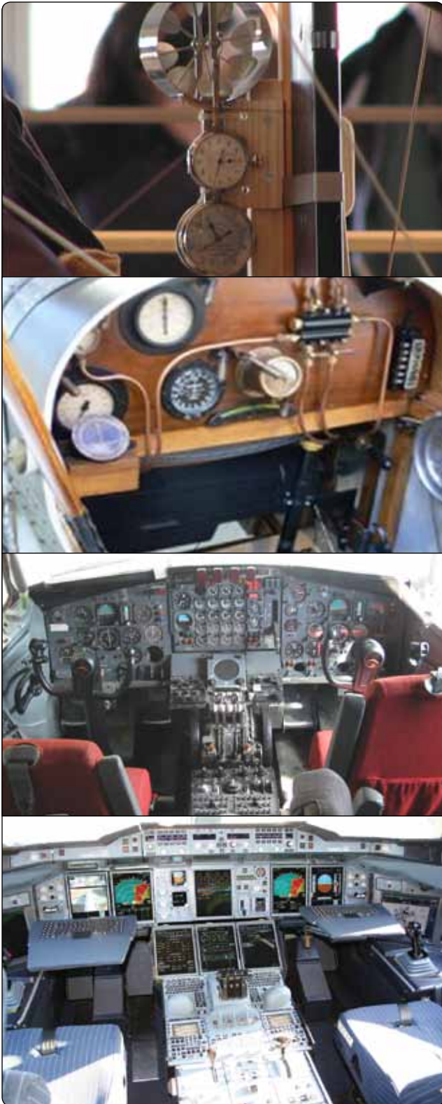
Figure 10-1. From top to bottom: instruments of the Wright Flyer, instruments on a World War I era aircraft, a late 1950s/early 1960s Boeing 707 airliner cockpit, and an Airbus A380 glass cockpit.
