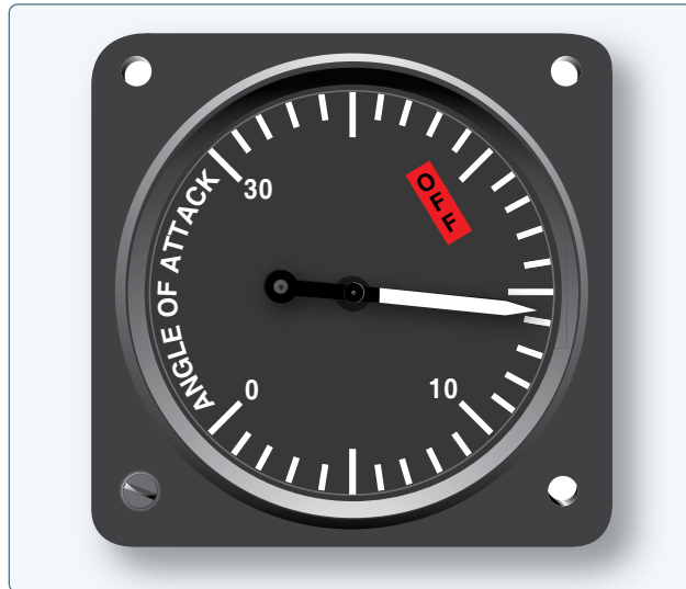
Figure 10-63. Angle of attack indicator.
