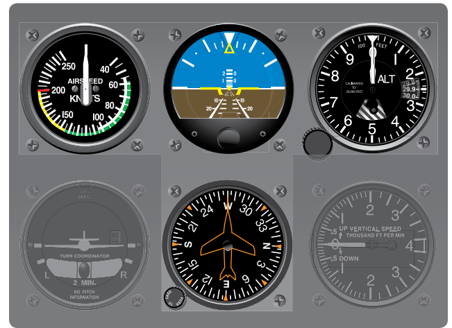
Figure 10-4. The basic T arrangement of analog flight instruments. At the bottom of the T is a heading indicator that functions as a compass but is driven by a gyroscope and not subject to the oscillations common to magnetic direction indicators.
