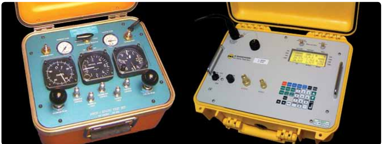
Figure 10-138. An analog pitot-static system test unit (left) and a digital pitot static test unit (right).
