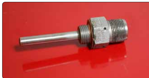
Figure 10-68. An electric resistance thermometer sensing bulb.
