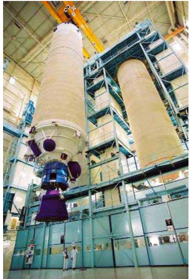
The Ariane 5 main cryogenic stage (EPC) in the integration dock at Les Mureaux, France, in course of preparation for containerization
