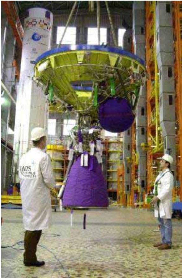
Ariane 5 ESC-A flight thrust frame at EADS-LV Les Mureaux, before departure for Astrium in Bremen.
