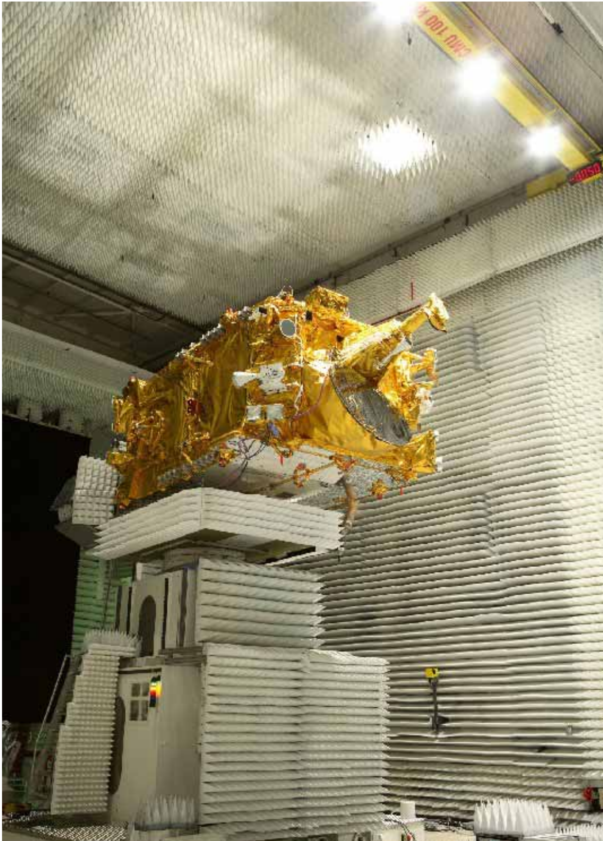
STAR ONE C2 anechoic chamber testing
