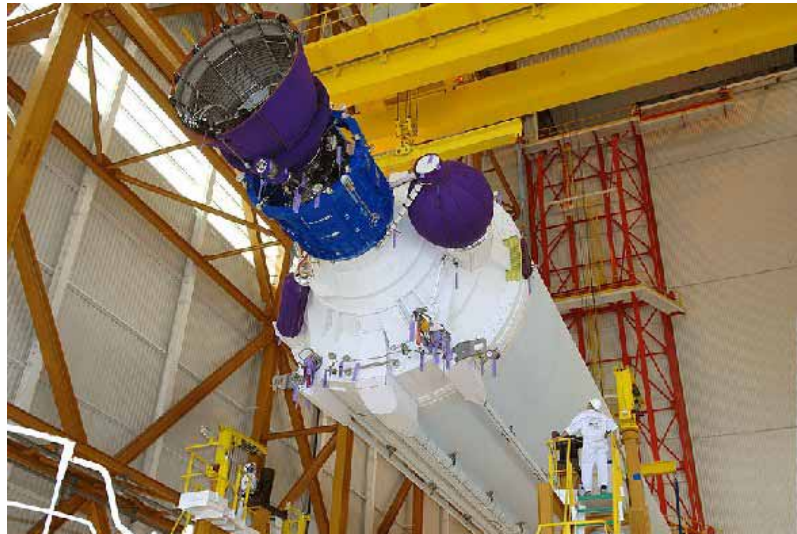
Kourou: depreservation and erection of the EPC in the BIL
