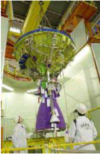
ESC-A thrust frame © EADS ST
