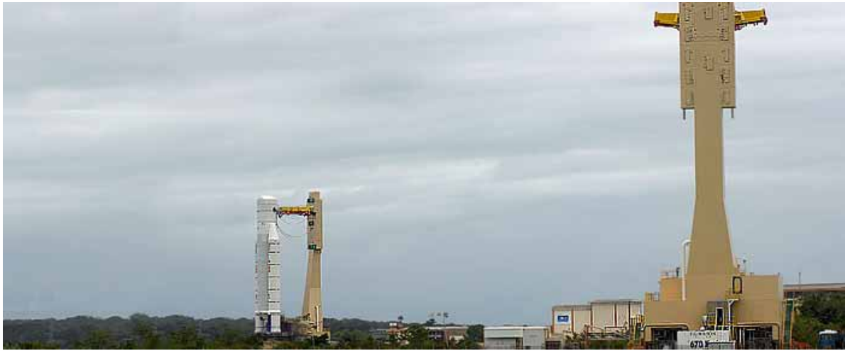
Kourou: transfer of the launcher from the Launcher Integration Building (BIL) to the Final Assembly Building. Foreground: table used for flight 181 and refurbished for the flight 182 campaign © ESA/ARIANESPACE/Service optique CSG
