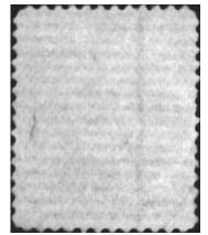
Laid lines as seen from the back VSC6000 photograph using spot fluorescence
