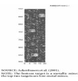
Fig. 6 – Images of landmines produced by GPR system
