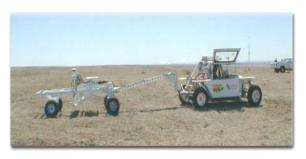
Fig. 3 Unmanned vehicle based landmine detection – Scheme 2
