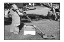
Fig. 7 - Prototype NQR Handheld Mine Detector
