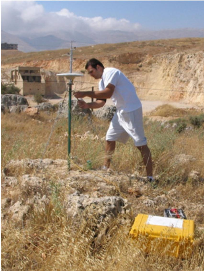
Figure 3.1: Fixed height mast with Zephyr antennae installed at HZRT.
