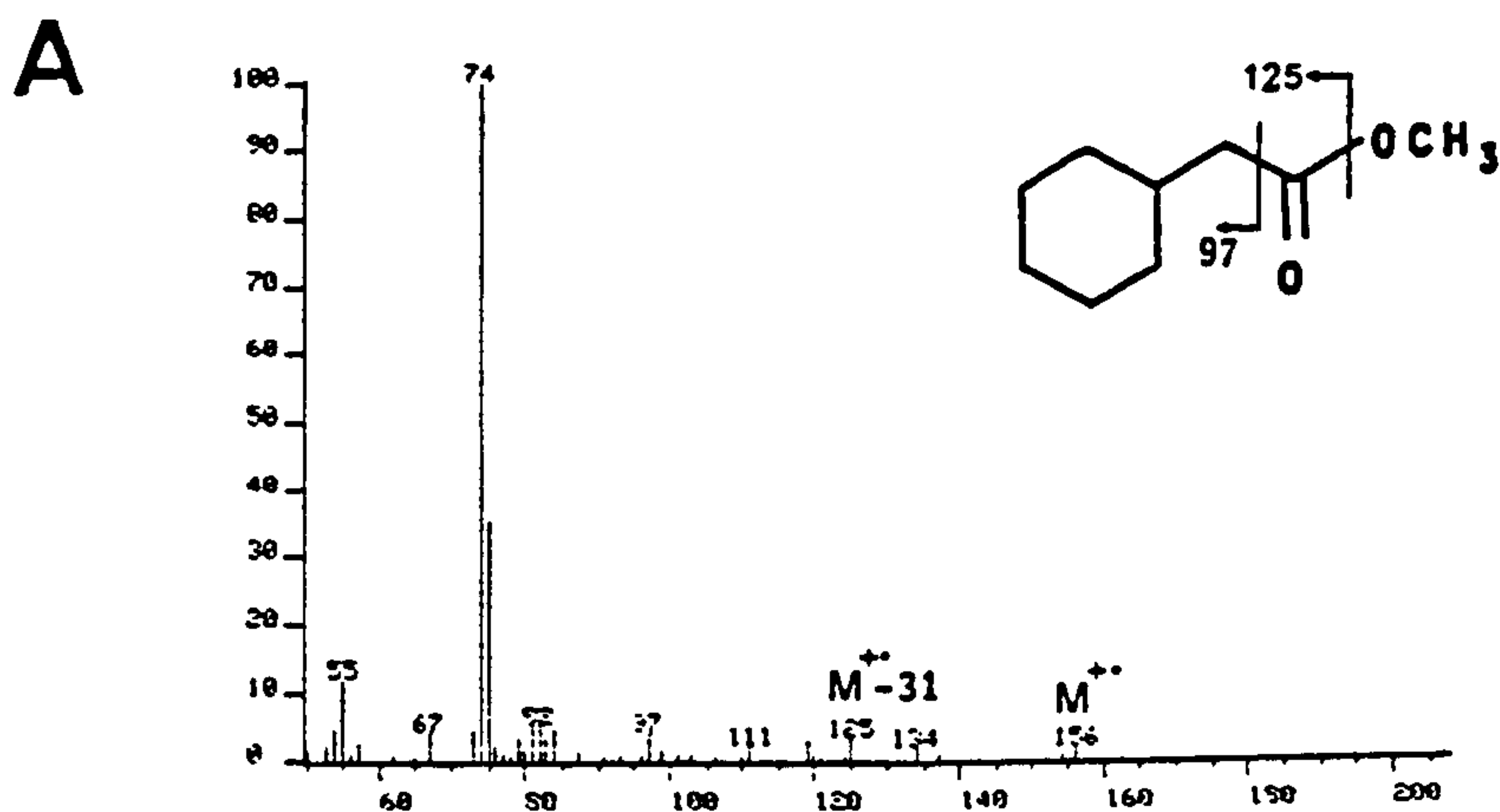
FIG 3.52 EI MASS SPECTRUM OF 2-CYCLOHEXYLETHANOIC ACID /METHYL ESTER IDENTIFIED AS A) AN ALIPHATIC UCM OXIDATION PRODUCT AND B) A PRODUCT OF OXIDATION OF 9-(2-CYCLOHEXYLETHYL)-HEPTADECANE
