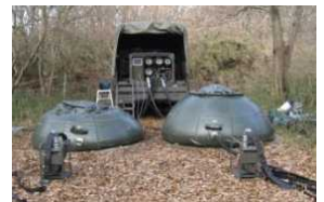
Water purification system that can turn seawater into potable water
