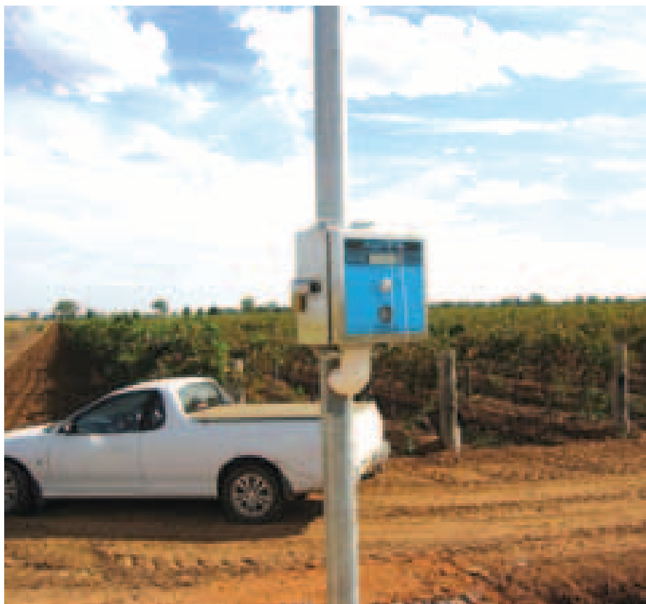
An ultrasonic water meter is used to measure irrigation water applied.
