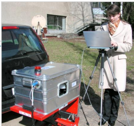
The portable detector of explosives and drugs, developed in the framework of the DVIN project
