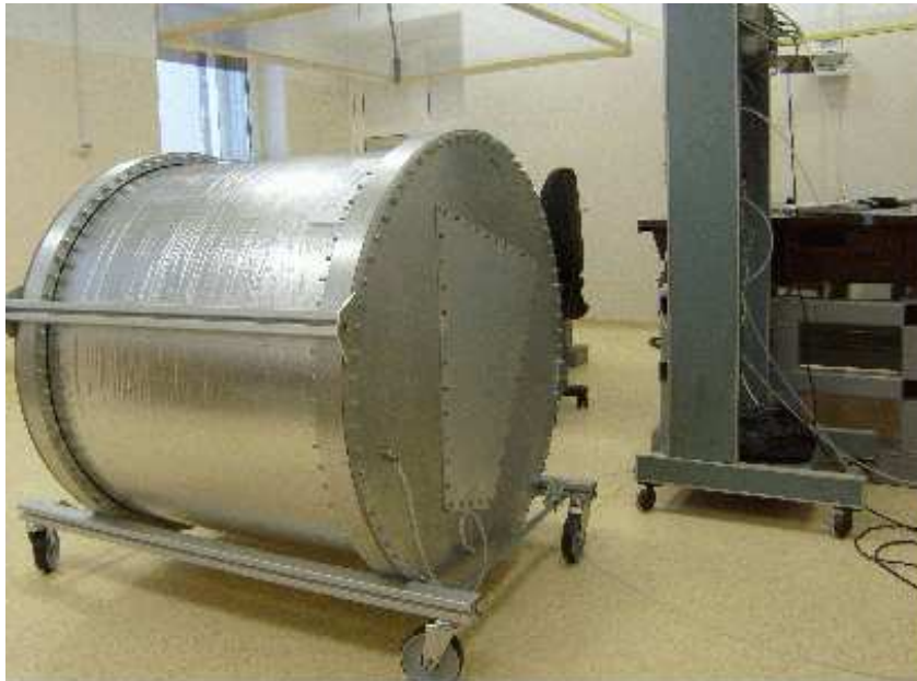
Fig. 2.49: The first prototype of the MPD TPC constructed in industry.
