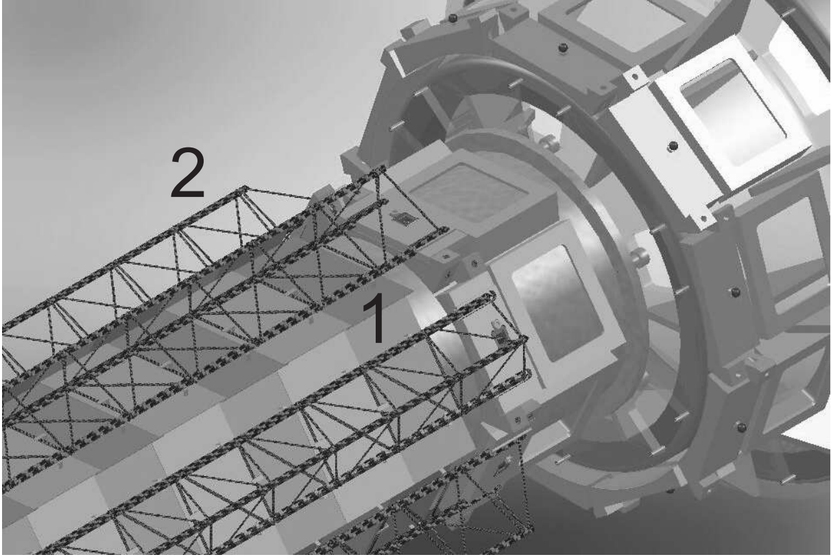
Fig. 2.57: The assembly of the first layer of the ITS cylinder part. Notations: 1 - silicon strip detectors; 2 - carbon fiber support (ladder).
