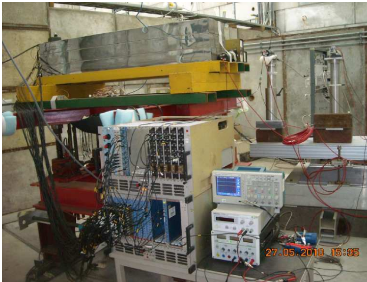
Fig. 2.133: Experimental setup in the May'2010 beam test (9 ZDC prototype modules are assembled on the top of the yellow-colored platform).
