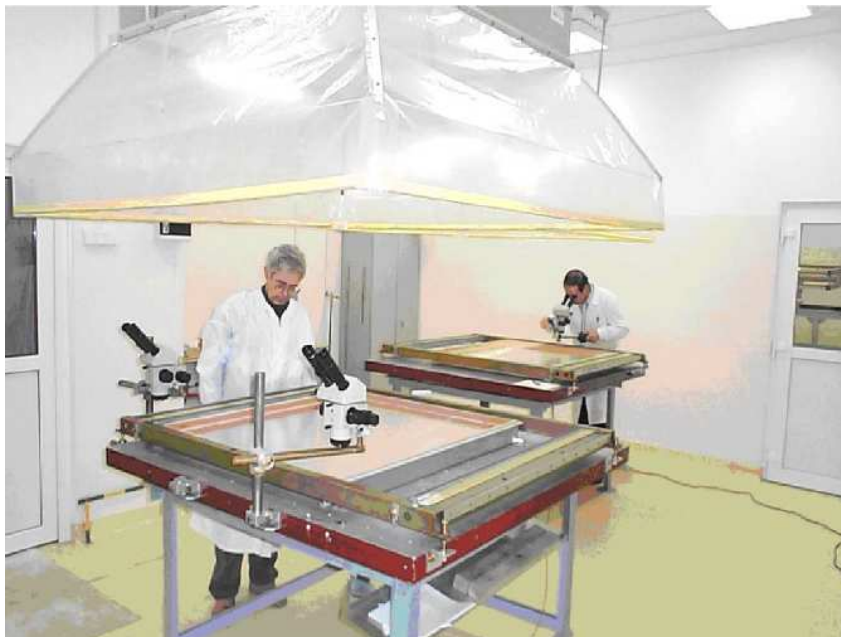
Fig. 2.47: Wire planes transfer on the chamber frames.
