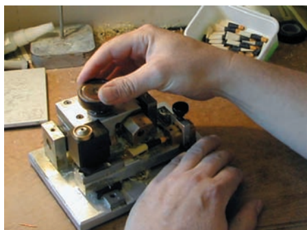
CHRIS APPS uses small steel forms (of the sort shown here) to help hand-fashion Australian Arundo donax cane into top quality chanter reeds.
