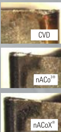
Worn inserts after 7 min of cutting
