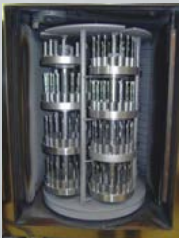
Coating of punches with DLC 2 in the \pi\text{C111}
