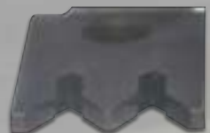
Wear on coated knife after tool life 5 \times L_m
