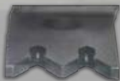
Wear on uncoated knife after tool life L_m = 10'000
