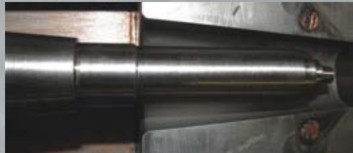
Coated tool by ALLWIN, Cr-Al-Si based coating Thickness: 2 to 3 \mu\text{m}
