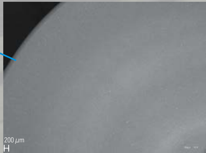
SEM micrograph of a lifter foot after a run with over 1000 miles
