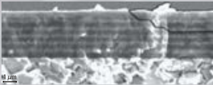
Multilayer for roughing: At dynamic load the cracks are absorbed at the borders of the sublayers.
