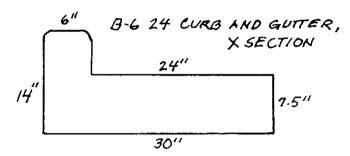
The concrete in the Fifteenth Street curb is 7.5 inches thick toward the center of the street and 13.5 to 14 inches high at the back or next to the grass on the parkway. The topmost part of the curb is 6 inches wide and the gutter part or pan extends for 24 inches making a total width of 30 inches as is later described in Section 8 in the 1923 Fifteenth Street specifications.
