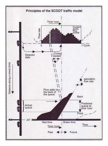
SCOOT has three optimisation procedures by which it adjusts signal timings - the Split Optimiser, the Offset Optimiser, and the Cycle Time Optimiser. These give SCOOT its name - Split Cycle and Offset Optimisation Technique. Each optimiser estimates the effect of a small incremental change in signal timings on the overall performance of the region's traffic signal network. A performance index is used, based on predictions of vehicle delays and stops on each link.
