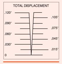
erating opposite to the normal side of its *tuning curve*. This happens when the tuning spring stiffness isn't great enough to achieve normal operation. In this case, you'll need to increase the stiffness until, when you adjust the tuning springs as outlined in rule 1 or 2, the adjustment begins to correct the tray's displacement. Then continue to tune the tray to the precise displacement your tray requires, again following rule 1 or 2.
