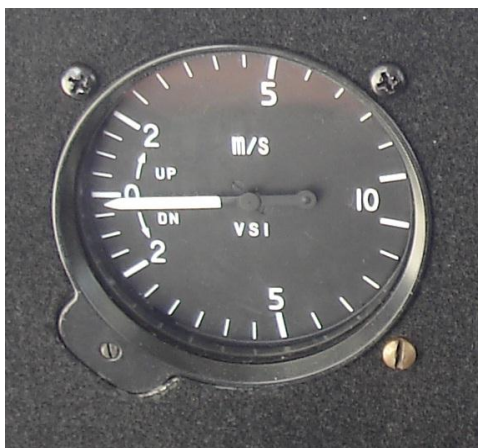
Fig 4.13. Variometru Ikarus C 42, Aerostar Festival
