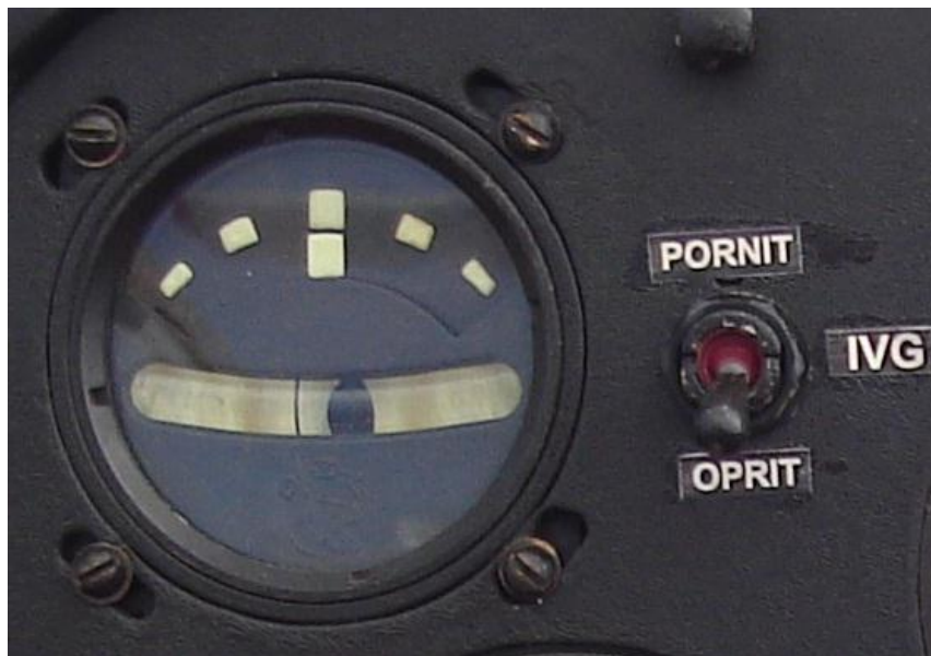
Fig. 4.16. Indicator de viraj si glisada planor IS 28 B2
