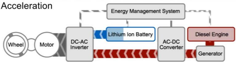
For further acceleration the Energy Management System will start the engine, and begins to blend the power to keep the engine operating efficiently.
