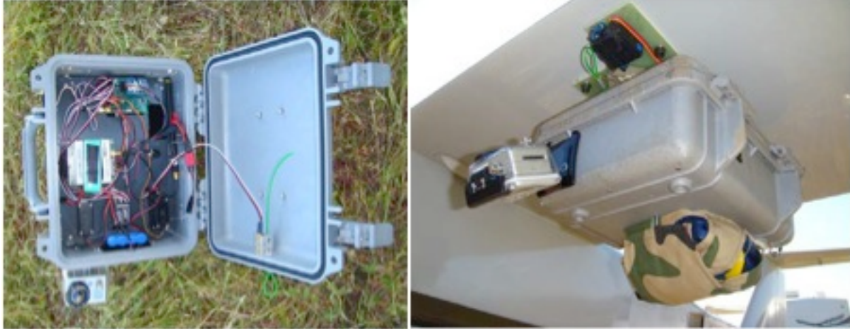
Figure 4. Snowflake GNC with the lanyard activated trigger in its lid (left) and release mechanism (right)
