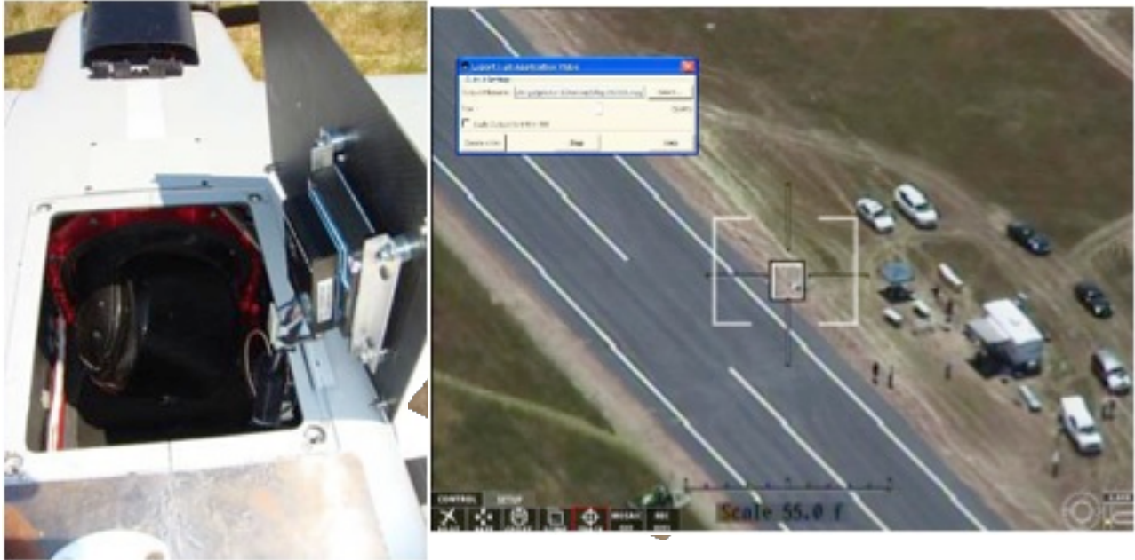
Figure 3. Microwave radio transmitter (left) and desired impact point chosen using TASE300 sensor (right)
