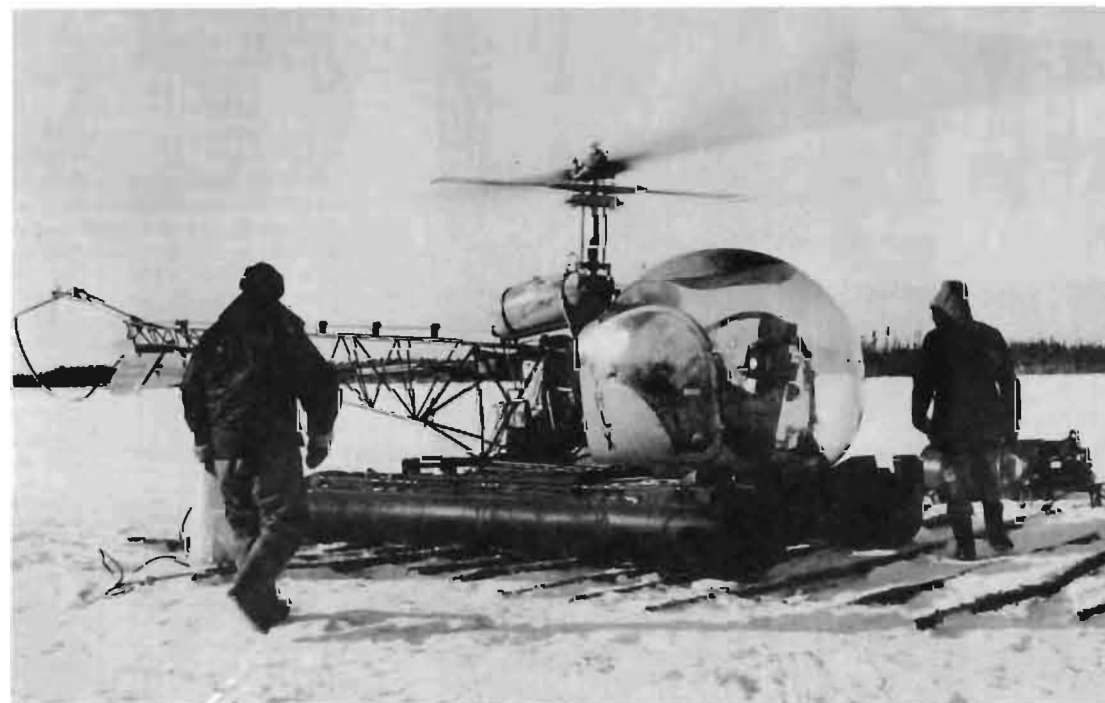
THEN AND NOW: Two old photographs (above) recall the difficulties of early surveyors when supplies and equipment were moved by canoe and pack. Today, left: an entire survey camp is delivered quickly by airplane. Below: a helicopter moves men easily from camp to work on the survey line. The platform prevents pontoons from freezing into snow.
