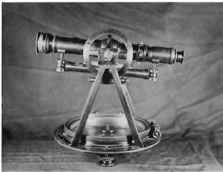
Top: Theodolite, circa 1830, used for sighting lines and measuring horizontal and vertical angles.
