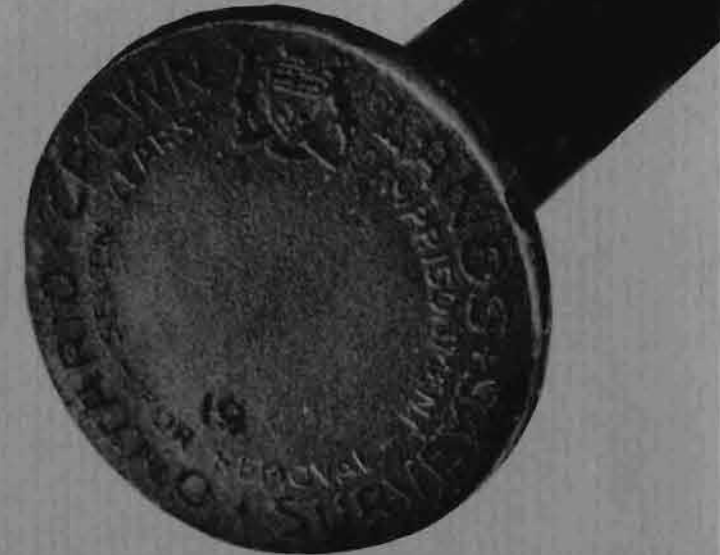
Crown Lands Rock Post (left) and Standard Iron Post (right) of the type used in government surveys in Ontario since 1920. The penalty for the removal of the Rock Post or the bronze plate on the Iron Post has been reduced from seven to five years of imprisonment. Below is the Crown Lands Short Standard Iron Bar, one inch square and 24 inches long, with "L&F" stamped on one side at the top to denote a Crown, Lands and Forests Survey. It was introduced in 1960, four years later than the Crown Lands Standard Iron Bar (bottom), one inch square and 48 inches long, which is driven through the bronze cap. BACK COVER: a typical example of the concrete monuments erected on the Ontario-Manitoba and Ontario-Quebec boundary lines.
