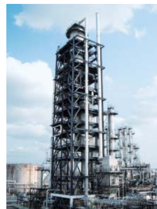
Facility located at the Mizushima Refinery in Okayama Prefecture for testing and research on the HS-FCC process
